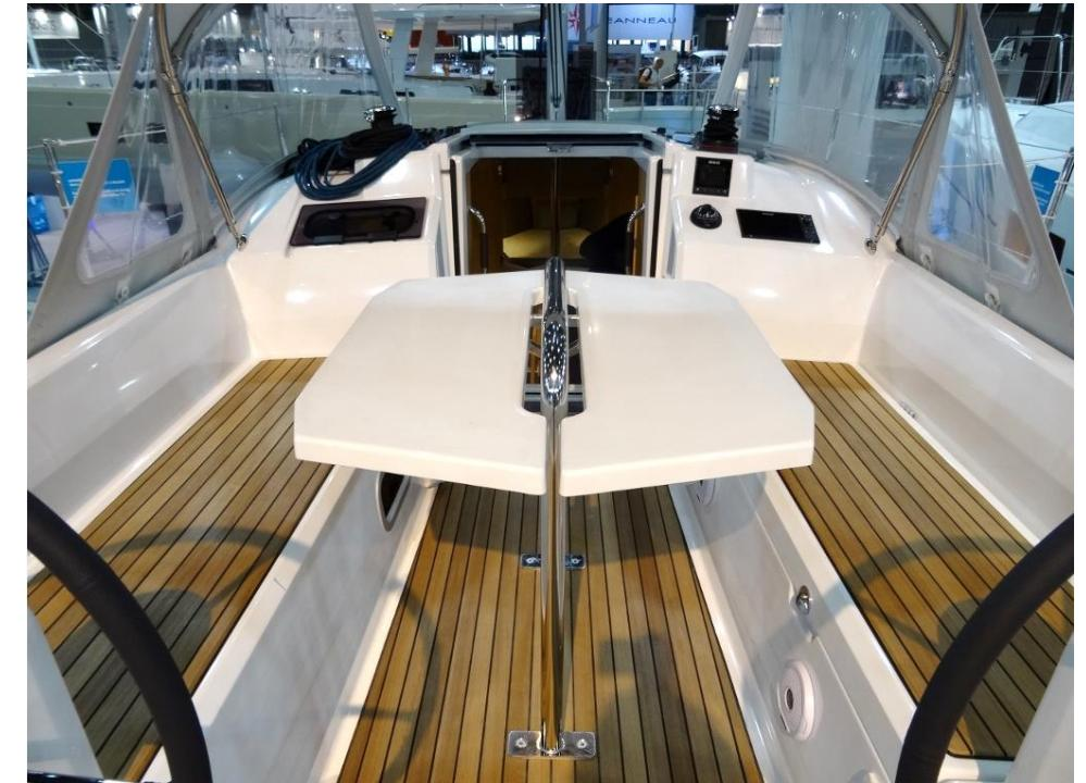
Natural solid wood decked aft platform with manual opening
