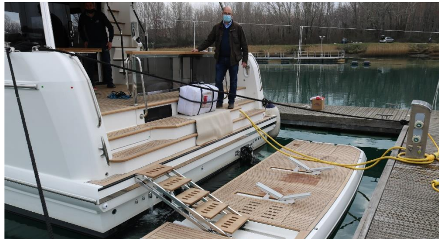
Hydraulic platform with integrated dinghy supports (400kg / 882lbs)
