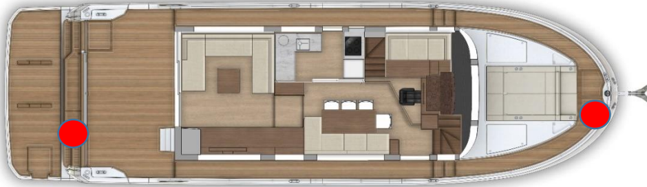
2x freshwater deck wash outlets (Transom & Bow)
