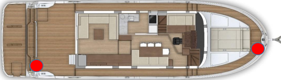
2x freshwater deck wash outlets (Transom & Foredeck)
