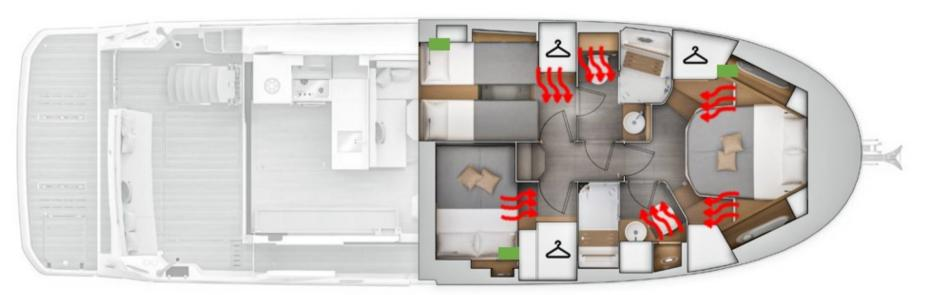
TOTAL DUCTED HOT AIR HEATING: 12KW TOTAL DUCTED HOT AIR HEATING: 12KW
