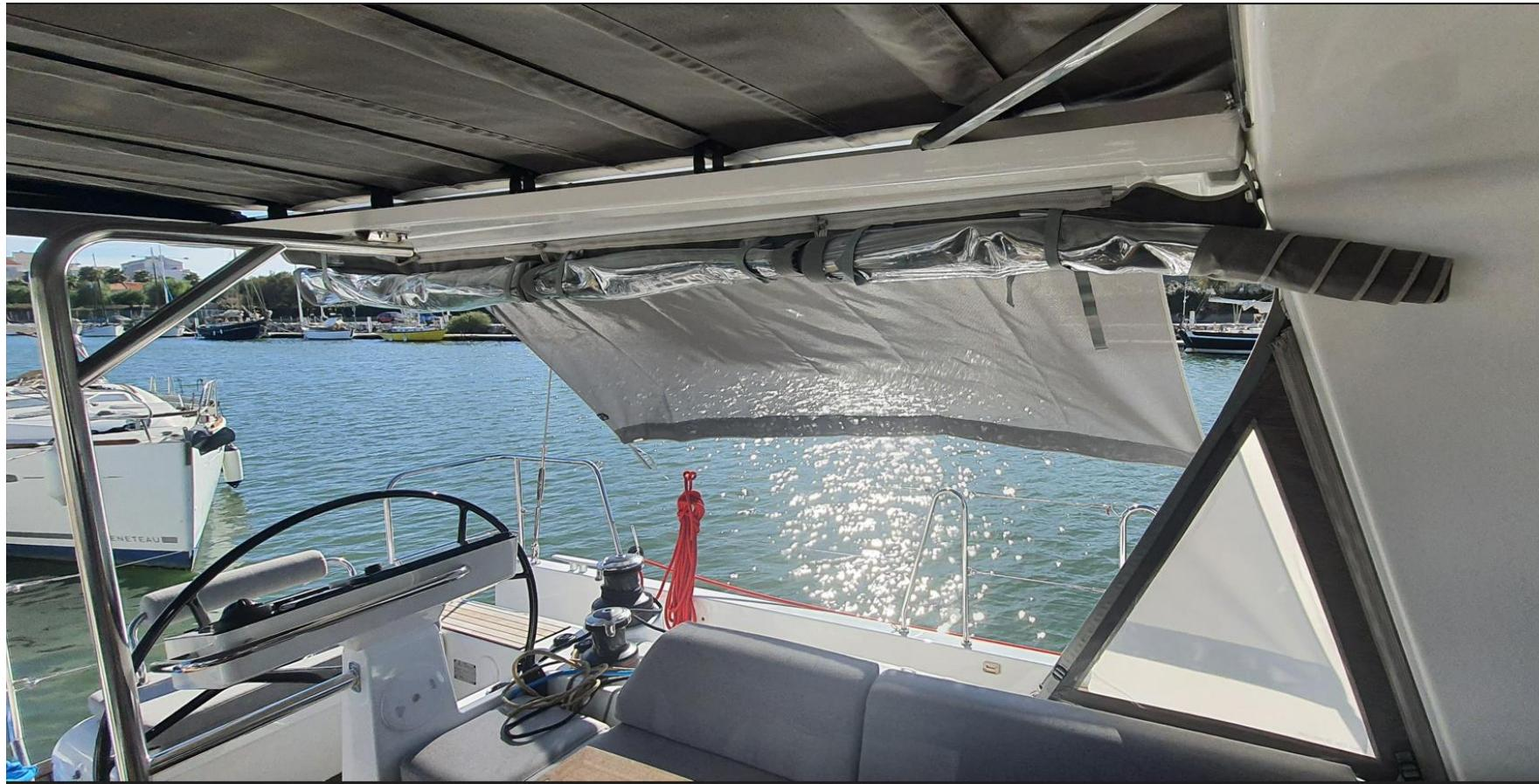
Possibility to roll up the closure along the bimini to open the cockpit.
