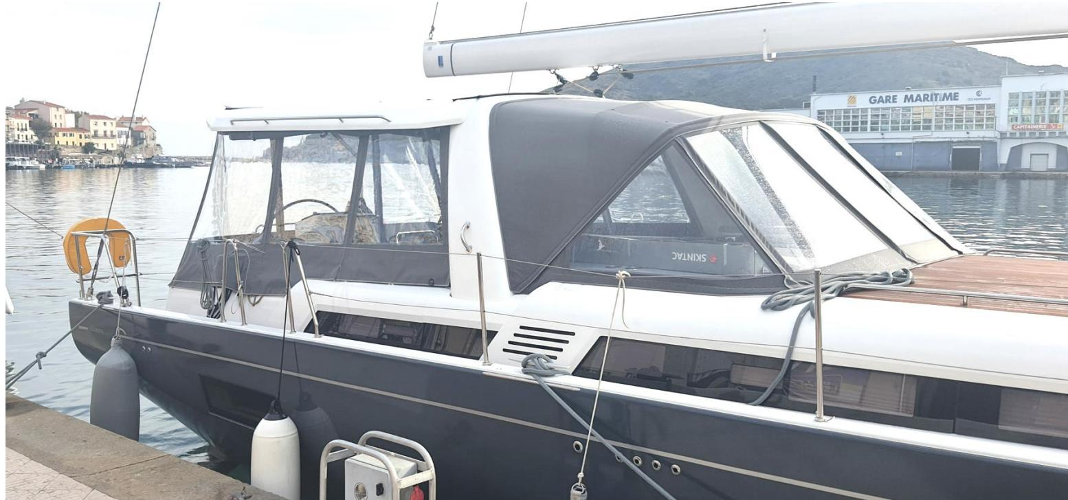
Complete closing of the bimini: sides and rear of the boat behind the helmsman seats.
