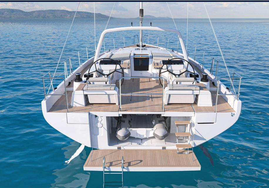
And since cruising goes hand in hand with anchorages the large bathing platform provides access to the tender garage, a must for a boat this size, capable of housing a 2.8 m jet-propelled tender. A system with double wires and guiding rollers makes for effortless launching and retrieval, promising active stopovers and lots of fun
